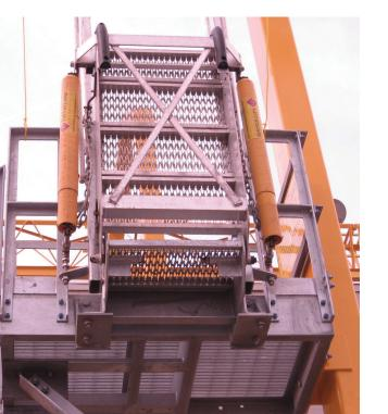
Diversified Fall Protection now offers hybrid fall protection. These hybrid systems include a platform of whatever length you require. Along the top of the platform, sliding gangways allow full access to your truck or rail cars at any position. The support columns for the platform double as footings for our overhead trolley rail fall protection. After installation of your platform, further fall protection can be added at any time with additional features.
