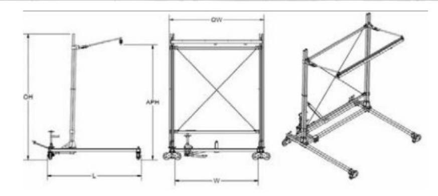
Mobile Horizontal Rail Systems may be fixed or adjustable in height. In addition, *an access* stair system with entrance platform can be incorporated to provide ground-up fall protection for your elevated work activities.
