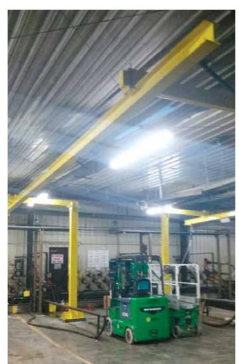
There are two important design considerations when determining a gallows system. First, the height of your rail cars or trucks establishes your fall clearance, which in turn determines whether a rigid or cable system is used. Second, the soil compaction around your tracks must be taken into account when designing the concrete foundations of the gallows.
