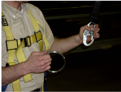
Figure 19 - Attach Steel Ring to SRL Snaphook
