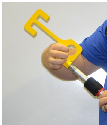
Figure 20 - Attach PTA to Extension Pole
