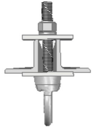
Figure 12 - Good Anchor Alignment
