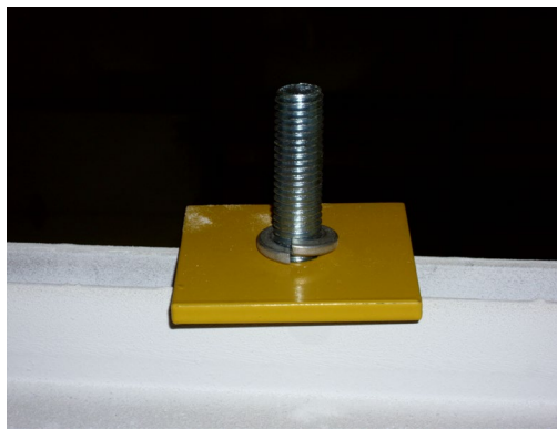
Figure 7 - Split Washer on Assembly
