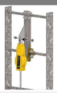
Secure the absorber onto the top anchor by the bolt and castellated nut provided with the absorber. Use the 19 mm wrench to rotate the nut until the split pin can be inserted through the hole in the bolt.
