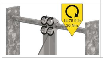
Evenly tighten the nuts using the deep socket to a torque of 14.75 ft lb (20 Nm).
