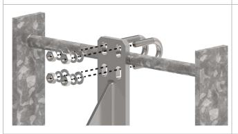
Secure the anchor onto the top ladder rung with the U-bolts and fixings from the top anchor fixing kit. Hand tighten nuts to hold anchor in position.
