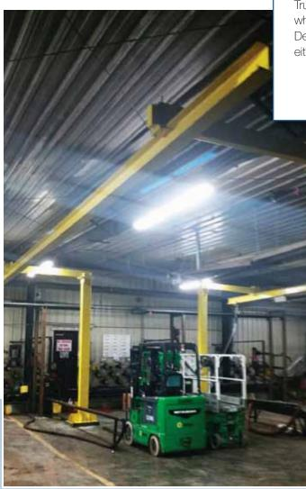
Gallows systems are used most often in outdoor applications that work with Trucking and Rail. Gallows systems always utilize overhead fall protection which reduces the fall distance since the anchorage is above the worker. Depending on the level of the working surface, gallows systems can be either rigid or lifeline systems.
