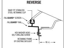
Shown below are some typical retaining frame profiles. Upon receipt of the quantity and dimensions of the clamp, Plasteco, Inc. can readily submit a quotation.
