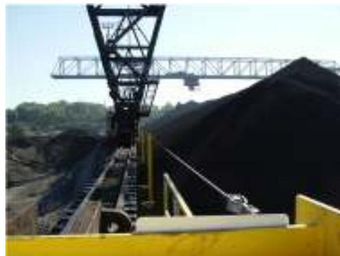
A horizontal lifeline runs across a crane rail provides safe inspection and maintenance at a mining facility.
