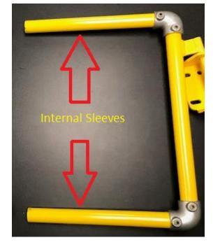
Next, with the internal sleeves loosely inserted into the elbow clamps, slide the "P"-Return over top of the sleeves until the desired overall length is achieved.
