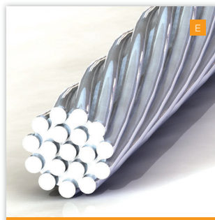
Cable 8mm (5/16") 1 x 19 316 stainless steel, high degree of stiffness allows free travel of attachment carriage and reduces cable deflections.
