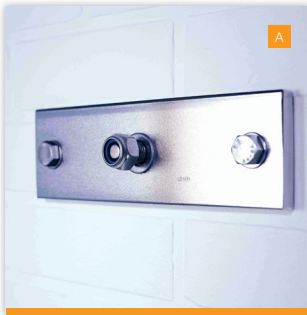
Wall Anchor Plate – 316 stainless steel, electro-polished. 50kN (11,205lbs) min breaking strength. 2 x M12 fixing holes.
