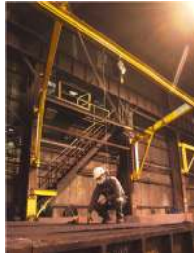
A worker using a rigid articulating trolley beam system while performing machine maintenance at a steel and foundry mill.
